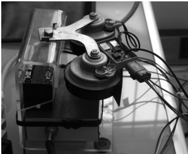
**Figure 1.** Multi Sound Horn (MSH) device provided by the FIAMM Group.
